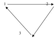
These types of sub tours have to be eliminated by the constraint. So, there introduce the constraint.
