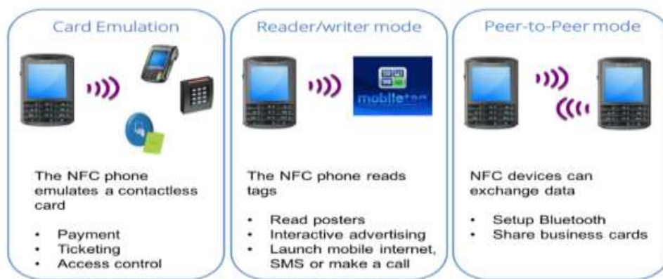
Figure 2 NFC operating mode(source (RFID 4u))
