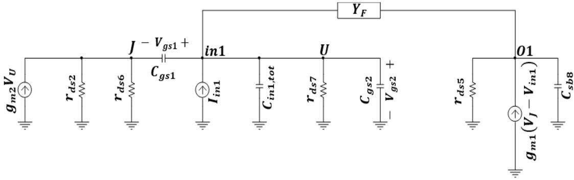
**Fig. 3: Small signal model (ac equivalent circuit) of the CG-CS input stage with active feedback.**
