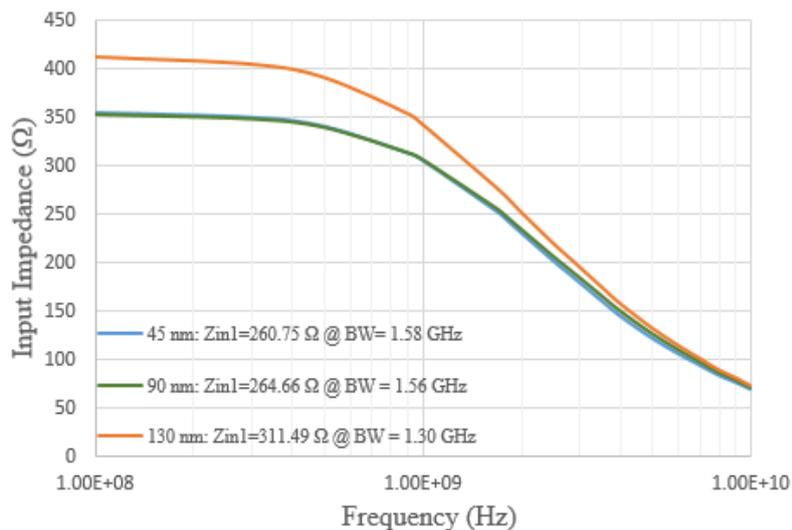
**Fig. 6: Input impedance frequency response at the channel length series (45 nm, 90 nm, 130 nm).**
