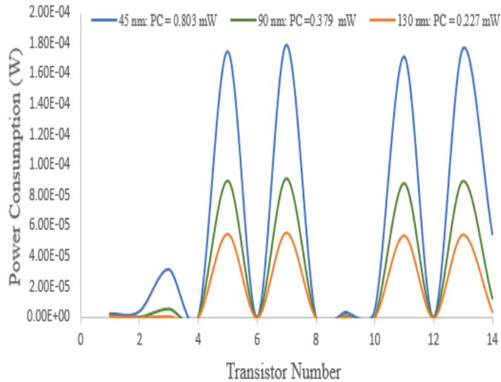
**Fig. 8:** Power consumption as per each transistor and total power consumption at the channel length series (45 nm, 90 nm, 139 nm).
