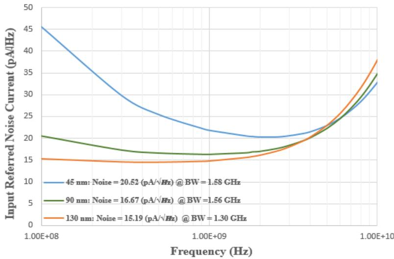
**Fig. 7:** Input referred noise current (spectral density) at the channel length series (45 nm, 90 nm, 130 nm).
