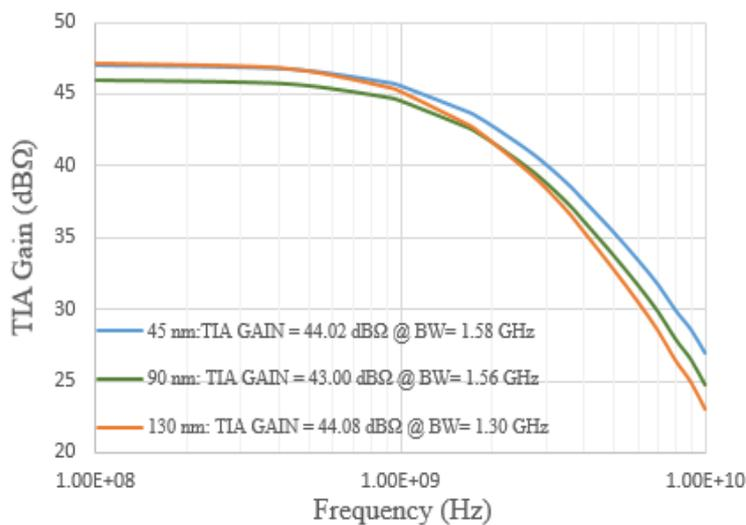
Fig. 4: Simulated TIA gain at the channel length series (45 nm, 90 nm, 130 nm) in (dBΩ).
