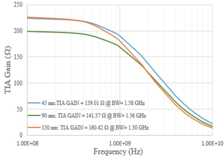
**Fig. 5: TIA gain at the channel length series (45 nm, 90 nm, 130 nm) in Ohm ( $\Omega$ ).**
