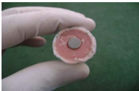
Figure (1): Show metal cylinder imbedded in acrylic with plastic mold.
