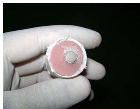
Figure (2): Composite application on metallic cylinder.
