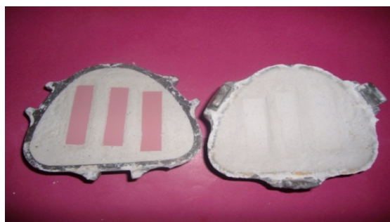
Figure (1) :Rectangular resin specimen for color testing.
