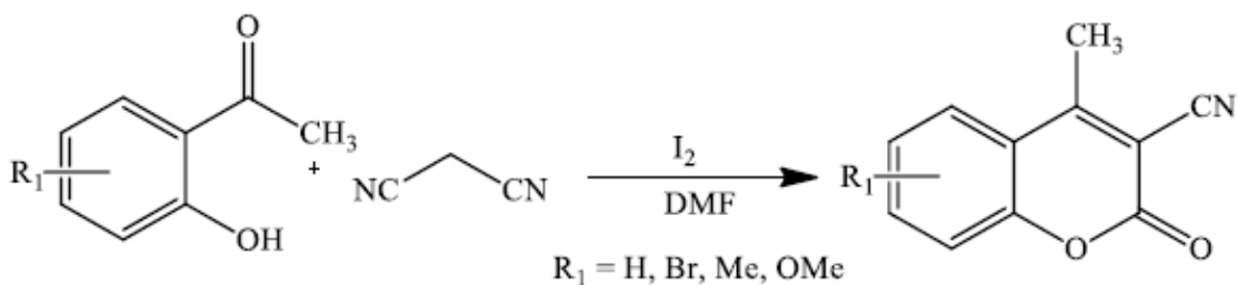
Scheme 15. A one-pot synthesis of 3-cyano-4-methylcoumarin compounds as described by Sharma and Makrandi.
