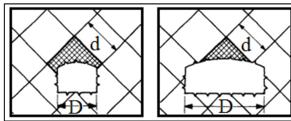
Fig.6. Influence of the span D on the stability in jointed rock (Kovari, 1979).
