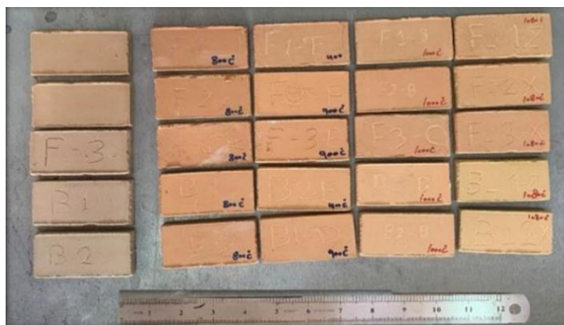
Fig. 6.the Fig. Shows Color Variation with Fired temperature
