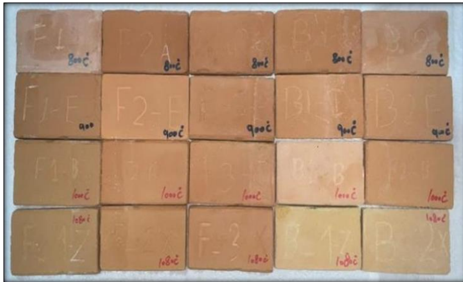
Fig. 9. The effect of efflorescence on the fired Bricks
