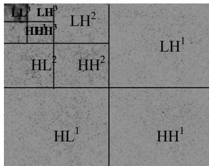
Fig.1: The structures of 2D DWT of third level
